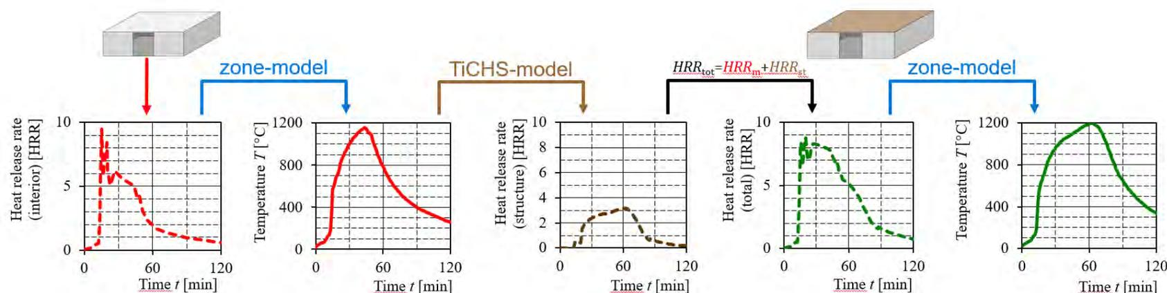
Fire load = movable fire load "+" structural fire load
