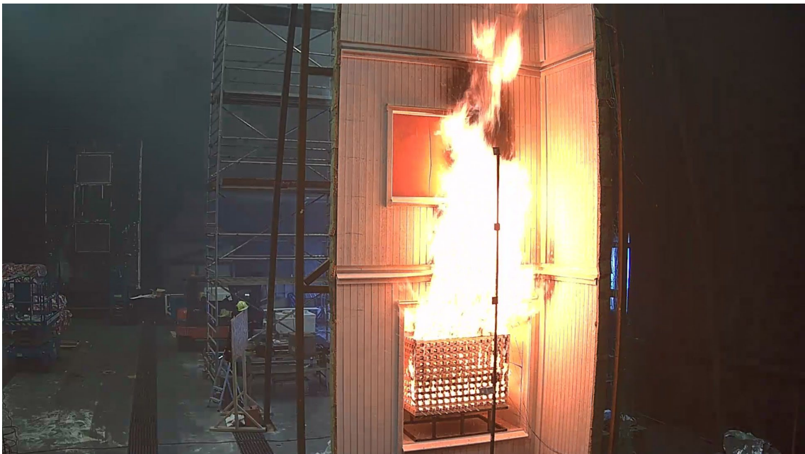
Photo 4 Draft proposed European test method, 2 minutes after first flames emerge out of the combustion chamber.
