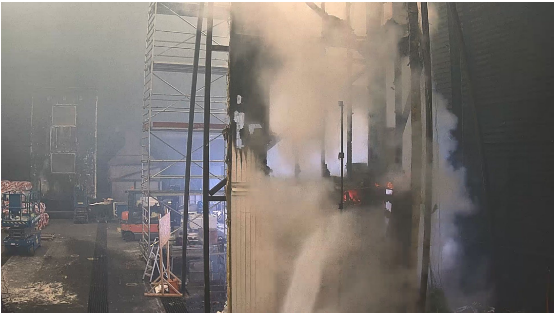
Photo 24 Draft proposed European test method after the wood crib and surface was extinguished with water.
