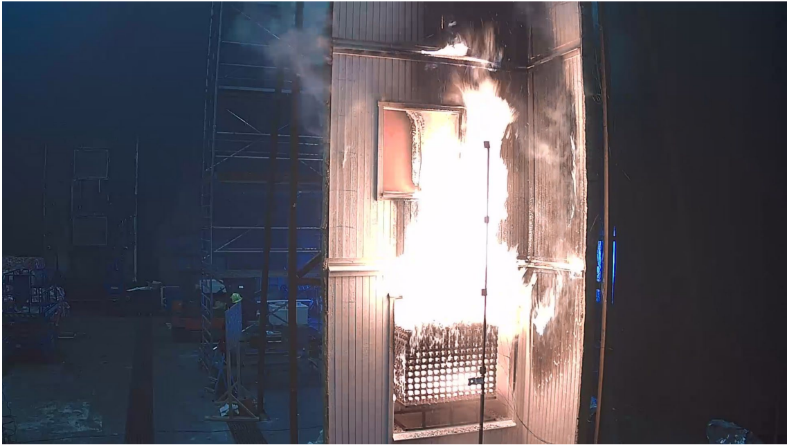
Photo 13 Draft proposed European test method, 12 minutes after first flames emerge out of the combustion chamber.
