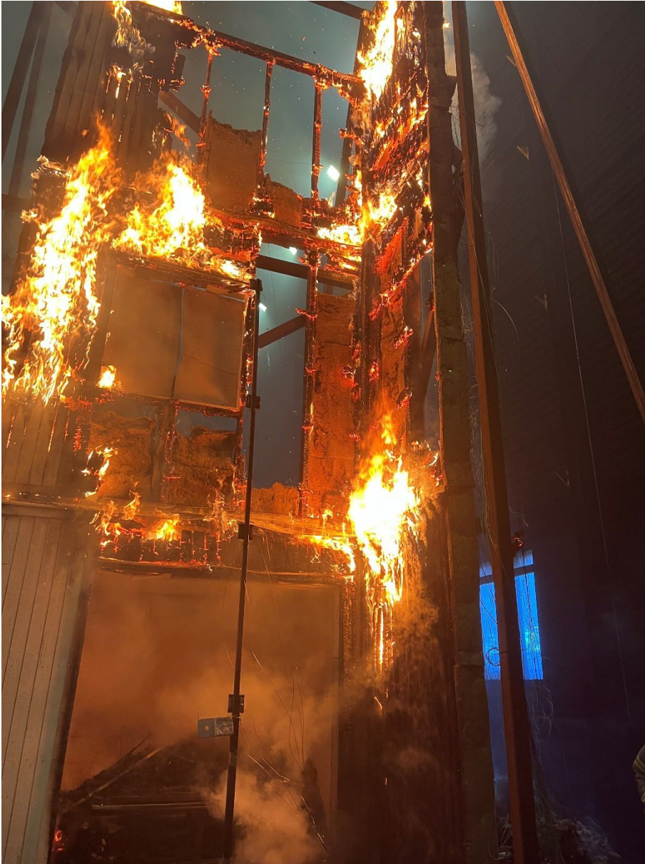
Photo B-9 Close up of the test specimen after the crib has been extinguished.
