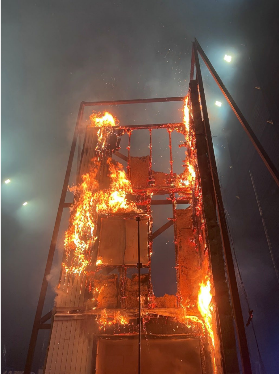
Photo B-10 Close up of the upper part of the test specimen after the crib has been extinguished.
