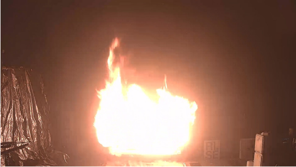
Photo 7 SP Fire 105, 6 minutes after first flames emerge out of the fire room.
