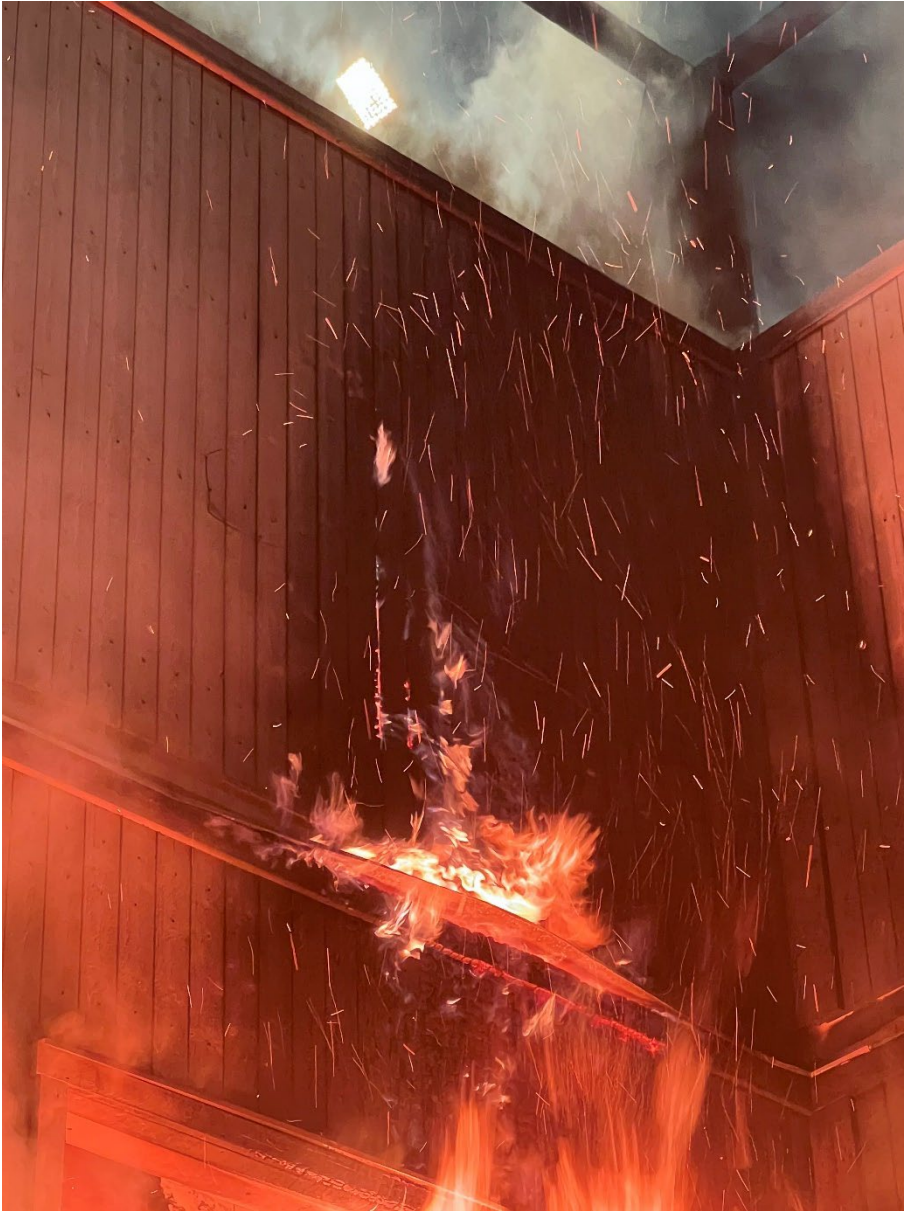
Photo B-5 Close up of the mid section flashing above the secondary opening halfway of the test
