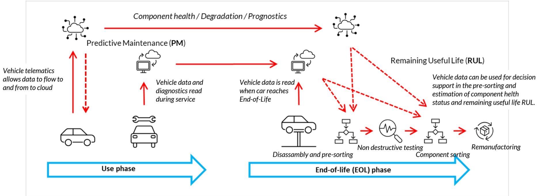
Illustrative schematic of sensor data flows during the **use phase** (through e.g. On-Board Diagnostics (OBD) port and telematics), and potential use (dashed arrows) for decision support in the pre-sorting and/or classification of the components condition during the disassembly and remanufacturing process at the **End-of-Life phase**.
