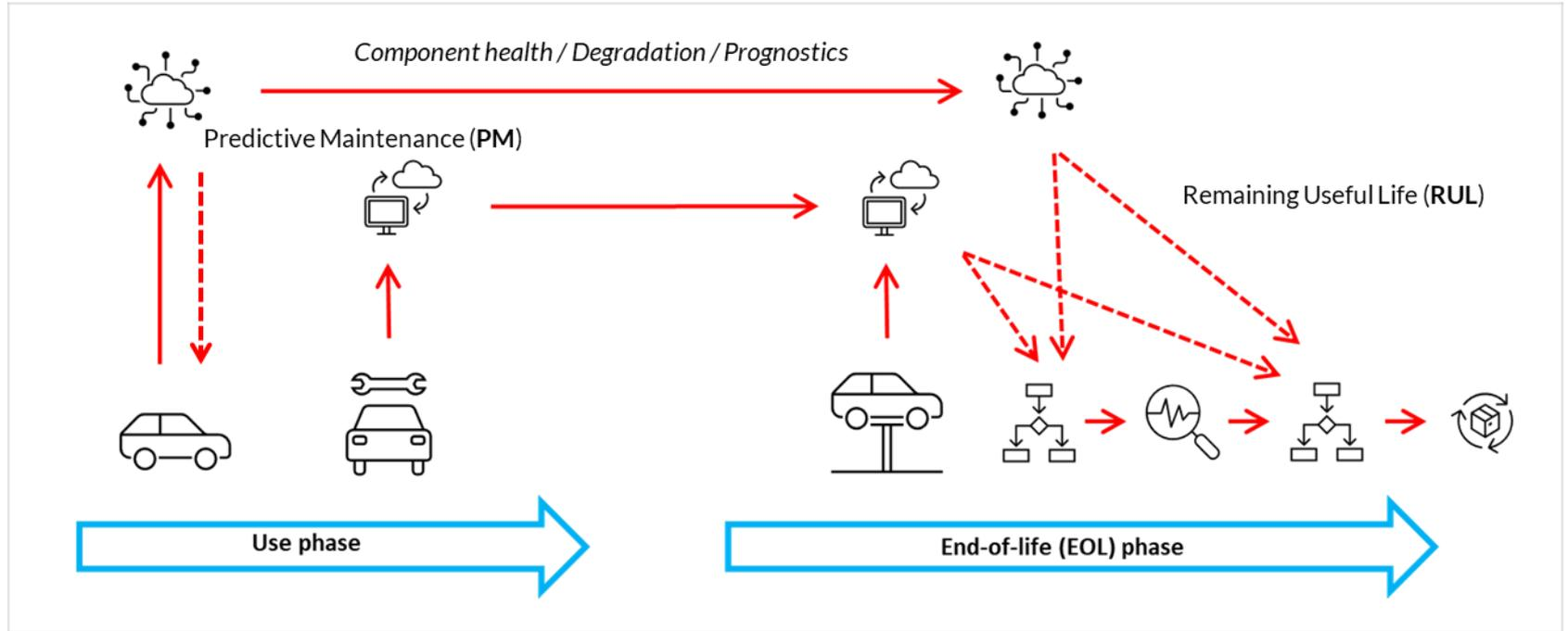
Illustrative schematic of sensor data flows during the **use phase** (through e.g. On-Board Diagnostics (OBD) port and telematics), and potential use (dashed arrows) for decision support in the pre-sorting and/or classification of the components condition during the disassembly and remanufacturing process at the **End-of-Life phase**.
