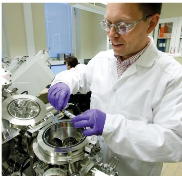
Samples ready to put into the XPS instrument for surface chemical analysis
