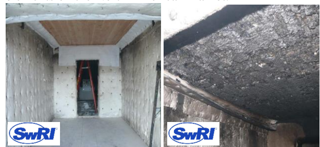
Figure 6: Impressions of compartment test with CLT (layer thickness 35mm) glued with PUR1 adhesive [16].
