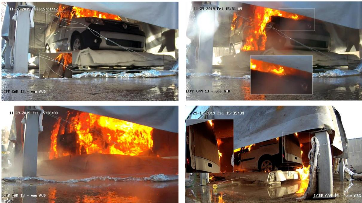
Figure 11: sequences of the light commercial vehicle fire; (top left hand side) fire developing at the front; (top right hand side) fire developing towards the rear of the vehicle with ignition of the right hand side plywood panels; (bottom left hand side) the fire is fully developed on the vehicle; (bottom right hand side) flame visible at the rear window.
