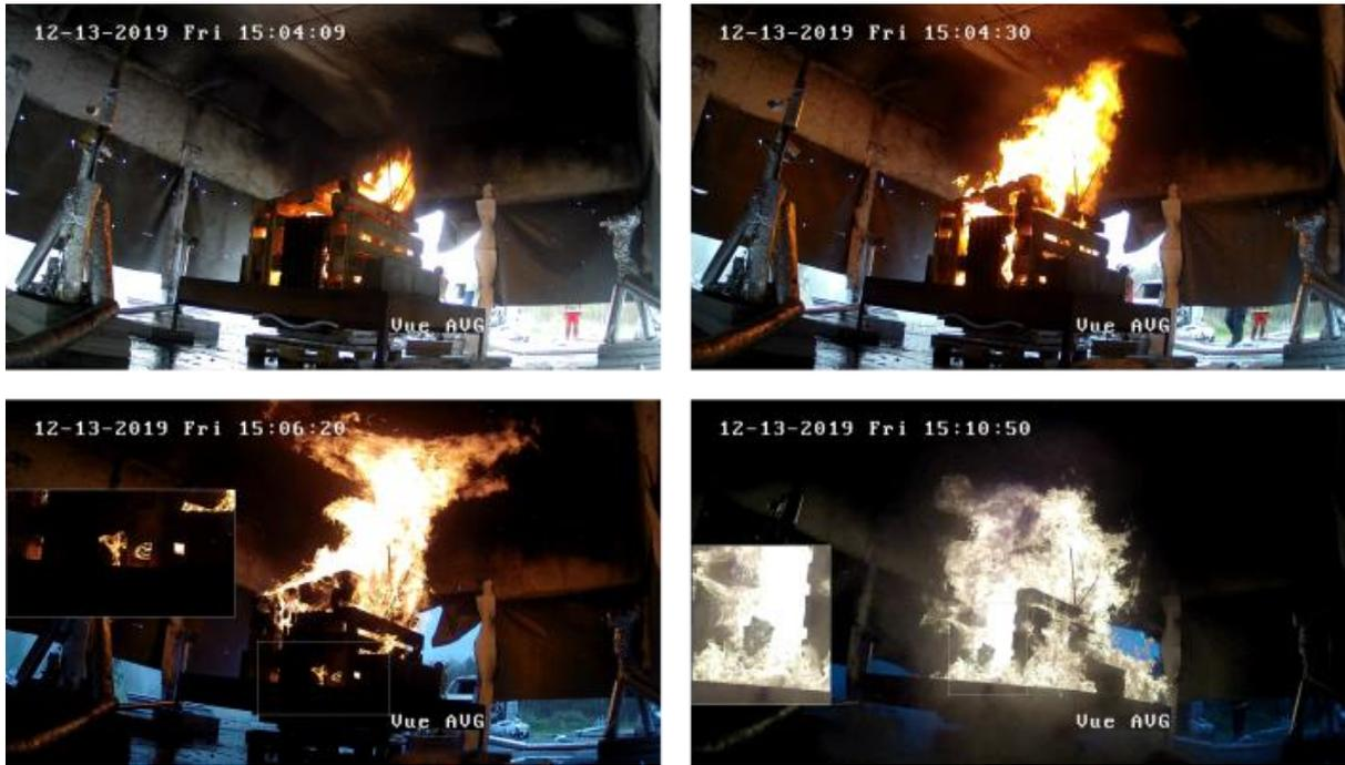
Figure 6: sequences of the load fire; (top left hand side) fire starting in the center; (top right hand side) fire developing in the center; (bottom left hand side) fire is fully developed and flame impacting the protective ceiling of large scale calorimeter; (bottom right hand side) flame enveloping the load .
