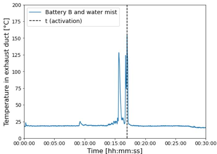
Figure 9 Temperature of battery fire test with active suppression by water mist
