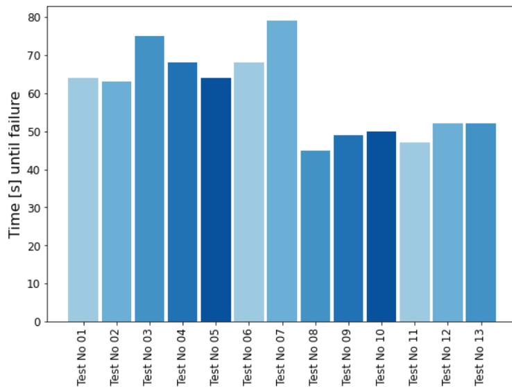
Figure 5 Duration of charging until ignition / failure of first battery cell
