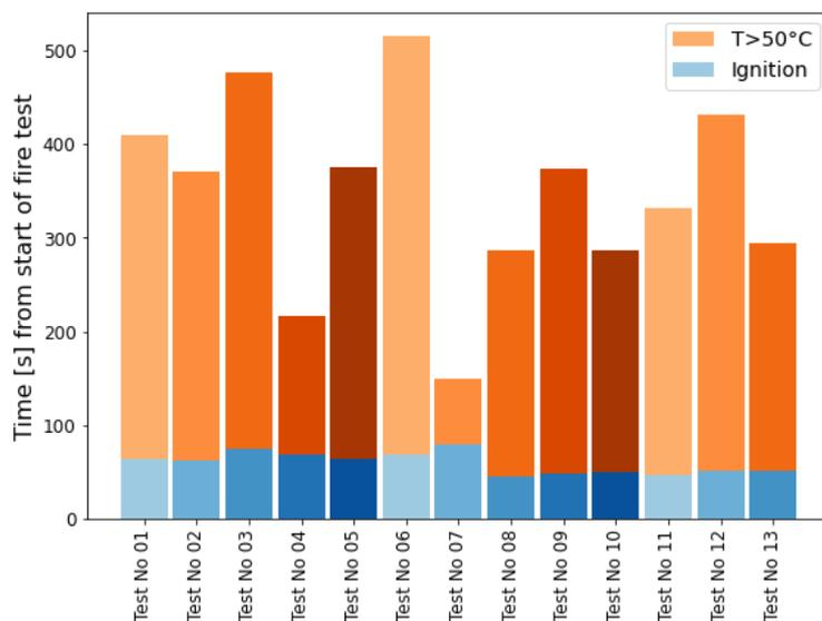
Figure 6 Duration until a mean value of 50 °C was measured inside calorimeter
