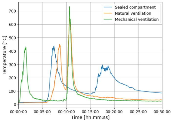
Figure 8 Time dependent-temperature resulting from Li-Ion module free burning tests with different ventilation conditions
