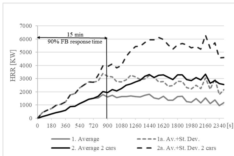
Fig 6. The average design fire heat release rate curves
