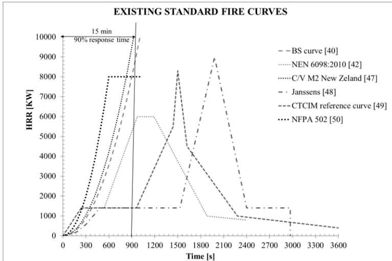
Fig. 1. Illustration of varying standards for fire heat release curves.
