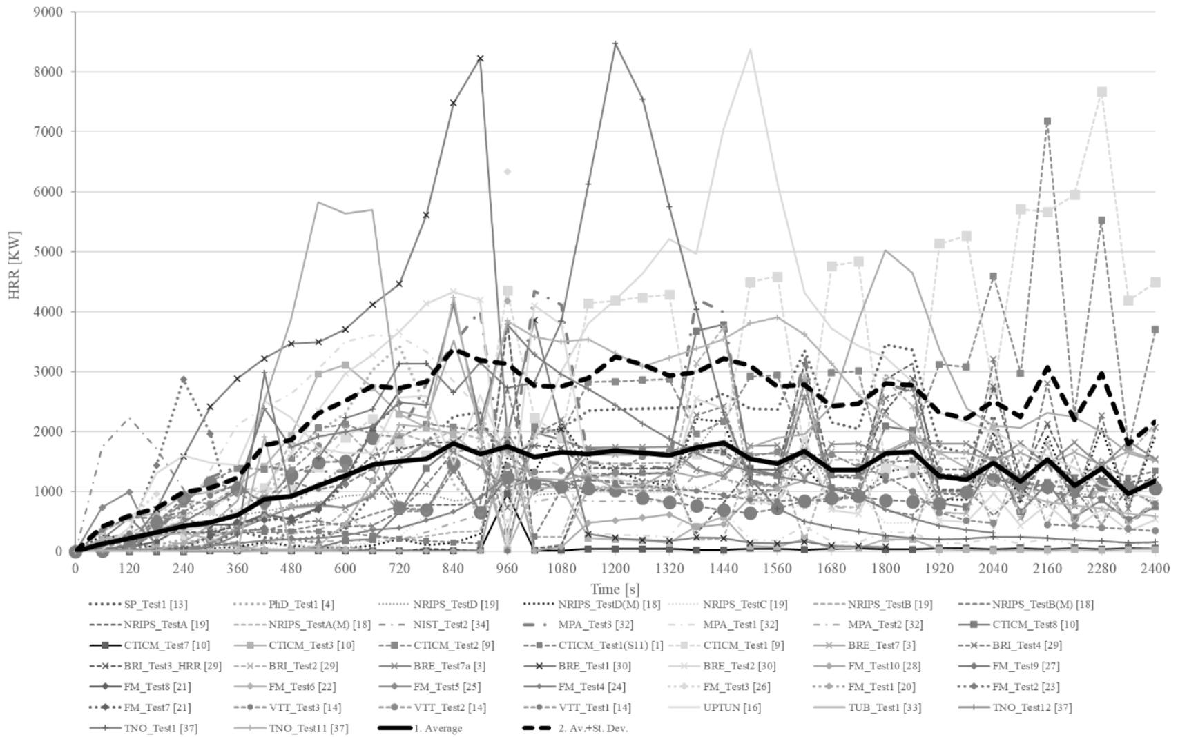
Fig. 5. Heat release rate curves of 44 real scale fire tests with their average curve and its positive standard deviation.
