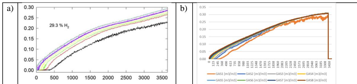
Figure 2. Hydrogen concentration increase a) experiment, b) CFD.
