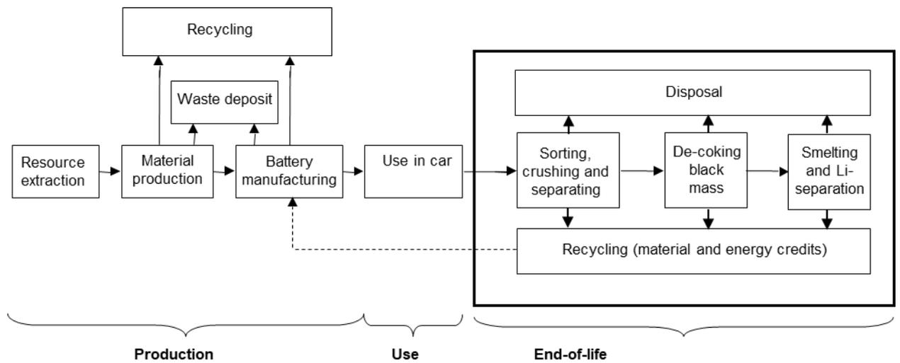
Figure 1 System boundary for lithium-ion study
