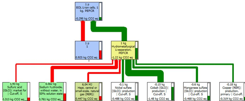
Figure 21 Climate impact of end-of-life recycling of lithium ion cells, PEFCR data, Swedish electricity mix
