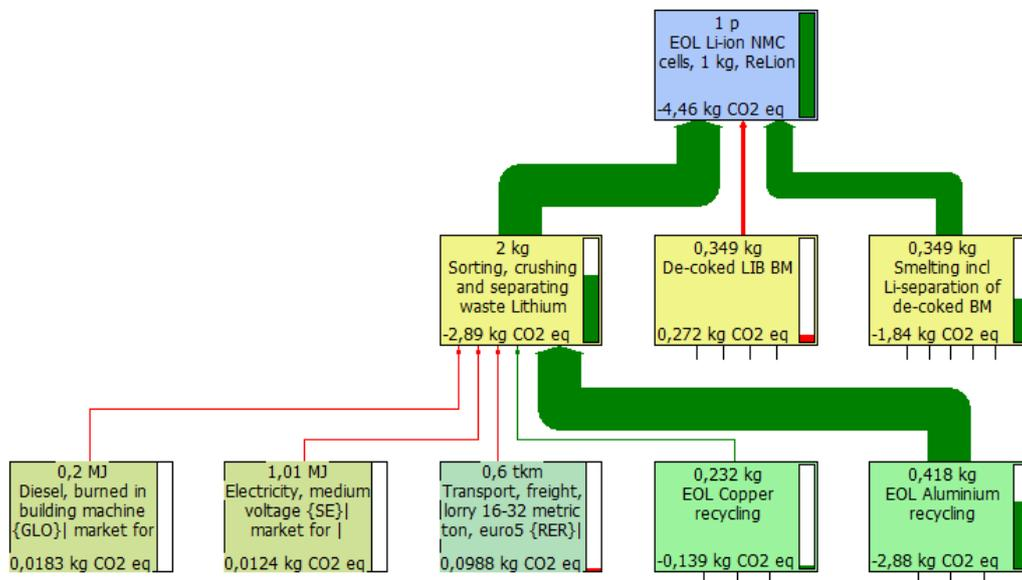
Figure 13 Climate impact of end-of-life recycling of lithium ion cells according to ReLion, sorting, crushing and separating, base case conditions
