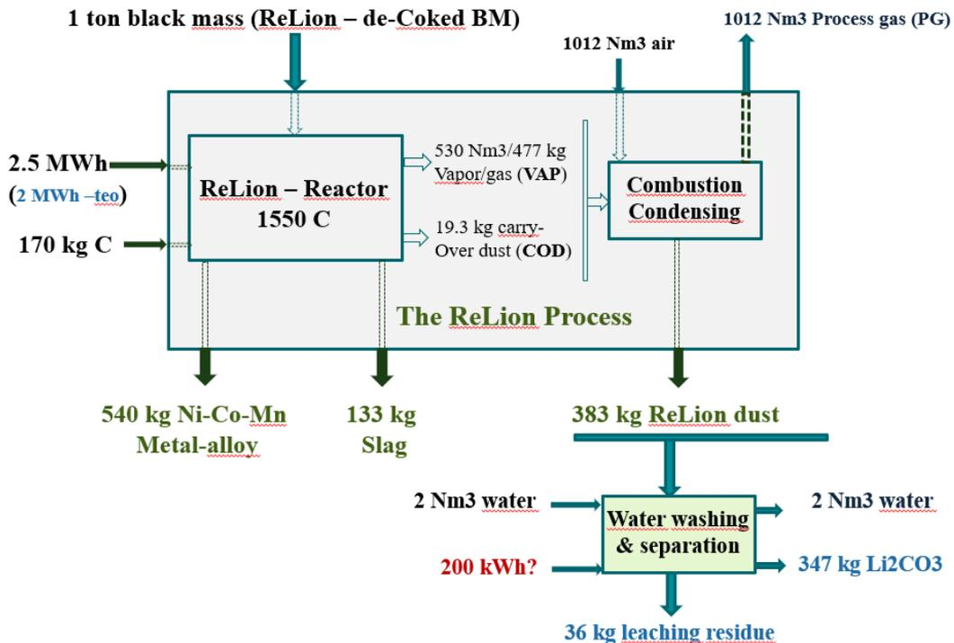
Figure 8 Step 2: Smelting reduction for Ni-Co-Mn recovery and Li-separation
