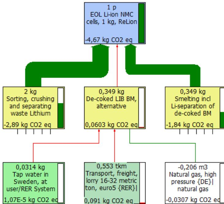
Figure 17 Climate impact of end-of-life recycling of lithium ion cells according to ReLion, decoking with air and water
