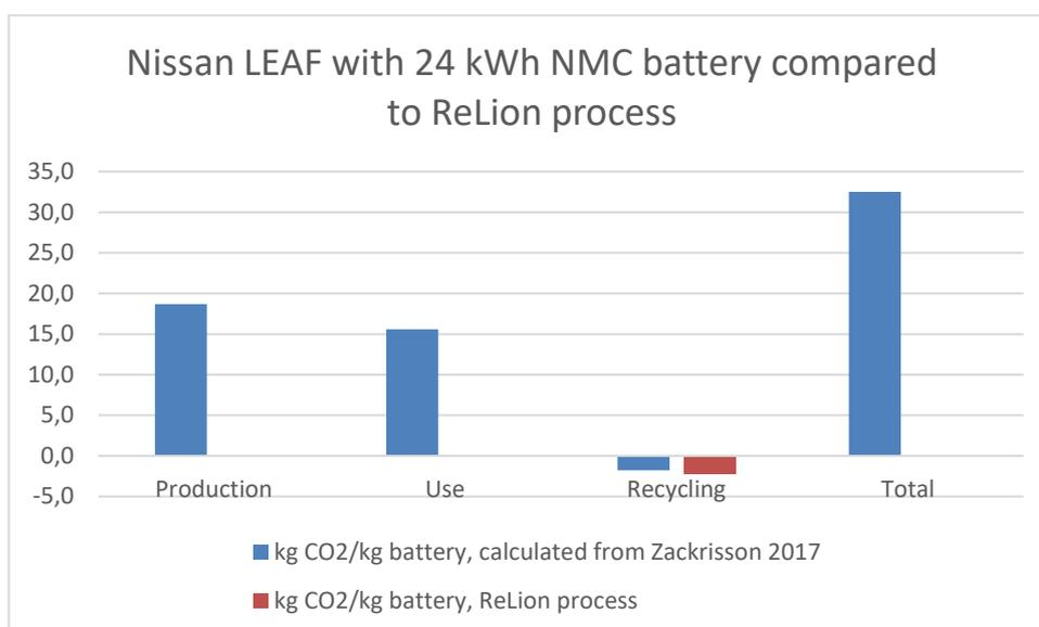
Figure 22 Nissan LEAF with 24 kWh NMC battery, life cycle climate impacts compared to ReLion process
