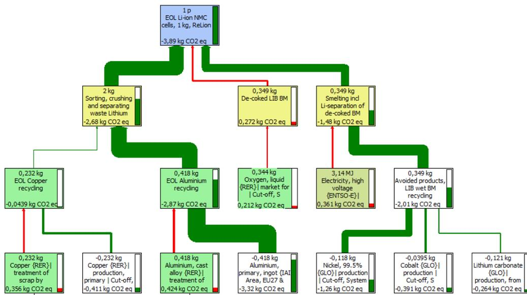
Figure 18 Climate impact of end-of-life recycling of lithium ion cells according to ReLion, European electricity mix
