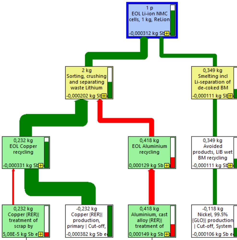
Figure 16 Abiotic depletion of end-of-life recycling of lithium ion cells according to ReLion, base case conditions, 5.3% cut-off
