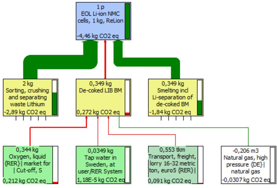
Figure 14 Climate impact of end-of-life recycling of lithium ion cells according to ReLion, decoking, base case conditions
