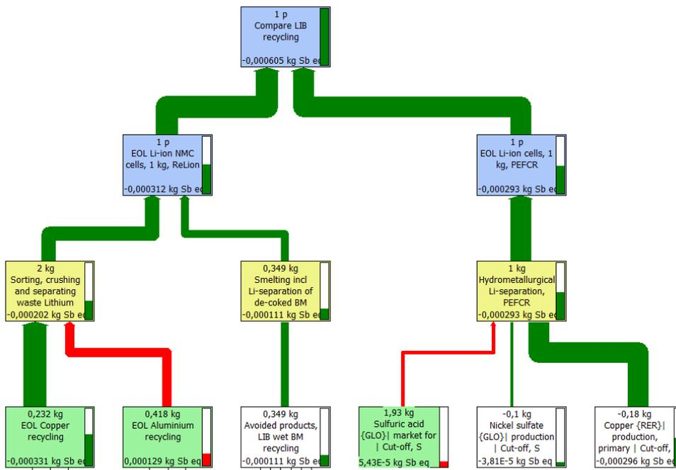
Figure 20 Abiotic depletion of end-of-life recycling of lithium ion cells. ReLion process compared with PEFCR data, European electricity mix. 3.5% cut-off
