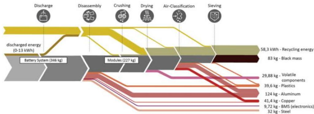
Fig. 16.7 Modeled energy and material flows from the LithoRec process
