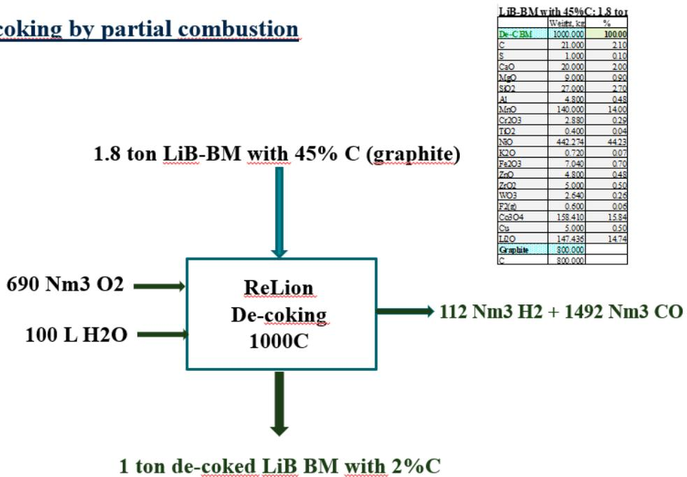
Figure 4 Step 1: decoke, separation of C from cathode material
