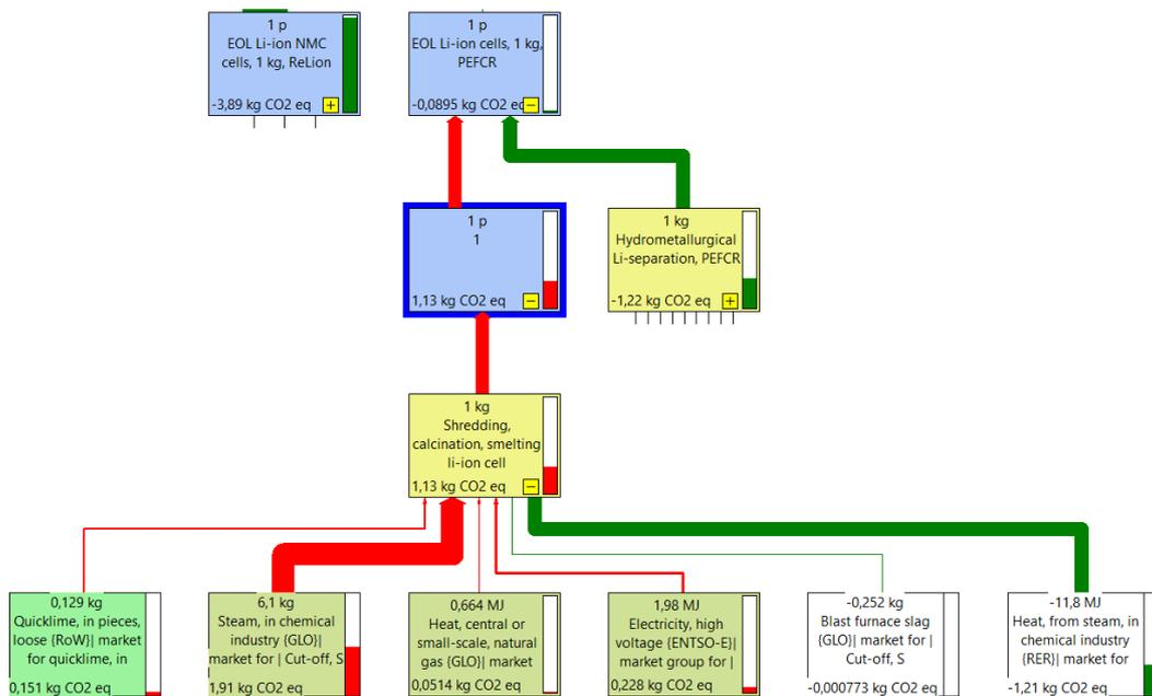
Figure 19 Climate impact of end-of-life recycling of lithium ion cells. ReLion process compared with PEFCR data, European electricity mix
