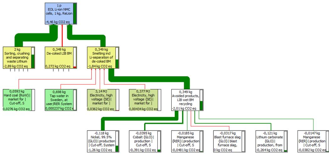
Figure 15 Climate impact of end-of-life recycling of lithium ion cells according to ReLion, smelting and Li-separation, base case conditions
