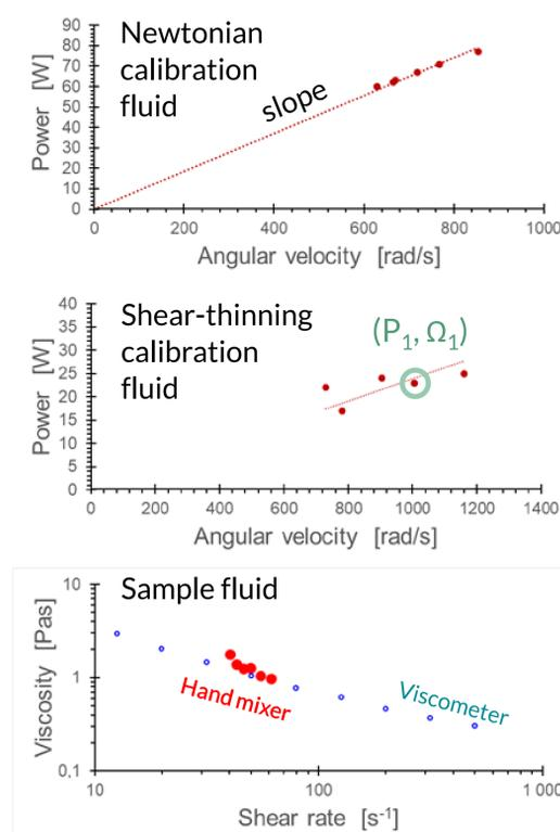
Step 1-3 for determining viscosity. Top: Newtonian fluid. Centre: Shear-thinning fluid. Bottom: Sample fluid data from the hand mixer and a viscometer as reference.
