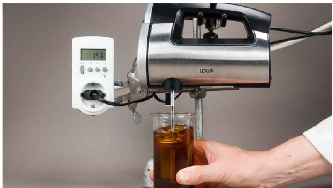
Setup for measuring viscosity using an electric hand mixer and an electric power meter.
