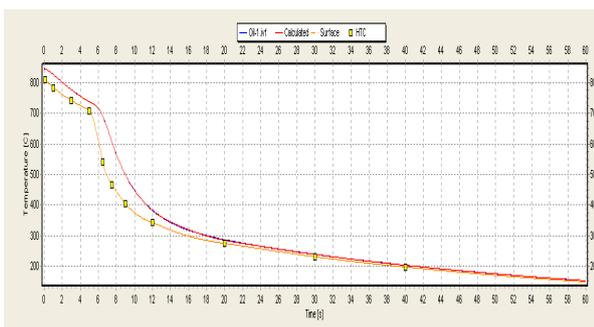
Diagram showing the measured (blue) and calculated (red) temperature versus time at the probe centre, and the calculated surface temperature versus time (orange) for a fast-quenching oil.
