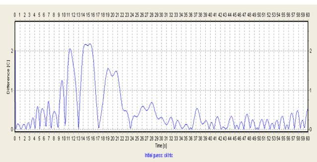
Diagram showing the difference between calculated and measured temperature at the probe centre. This is a tool for evaluating the accuracy of the calculation.
