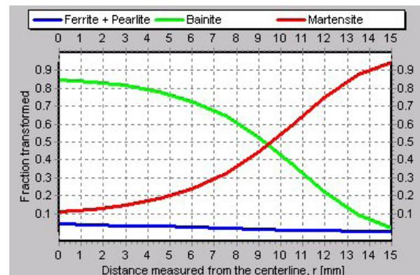
Calculated microstructure distribution in a cross-section of the steel specimen to the left.
