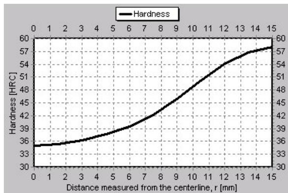
Calculated hardness distribution in a 30 mm dia. C45 steel specimen, quenched in a polymer quenchant at 28 °C.
