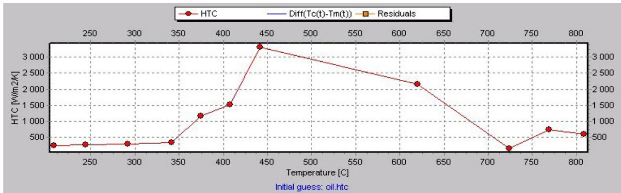
Calculated heat transfer coefficient versus surface temperature of an ISO 9950 standard test probe (12.5 mm dia. x 60 mm, made of Inconel 600), quenched in a fast quenching oil.
