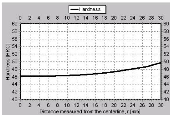
Calculated hardness distribution in a 60 mm dia. 34Cr4 steel specimen, quenched in a fast oil at 70 °C.
