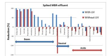
Reduction of pharmaceutical residues in spiked MBR effluent, measured with LC/MS/MS
