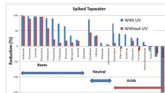
Reduction of pharmaceutical residues in spiked tap-water measured with LC/MS/MS
