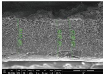
Membrane thickness shown in a cross section of the membrane.
