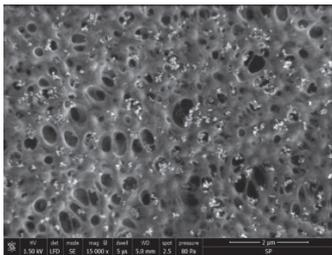
SEM image of the membrane showing the photocatalysts on the PVDF membrane.
