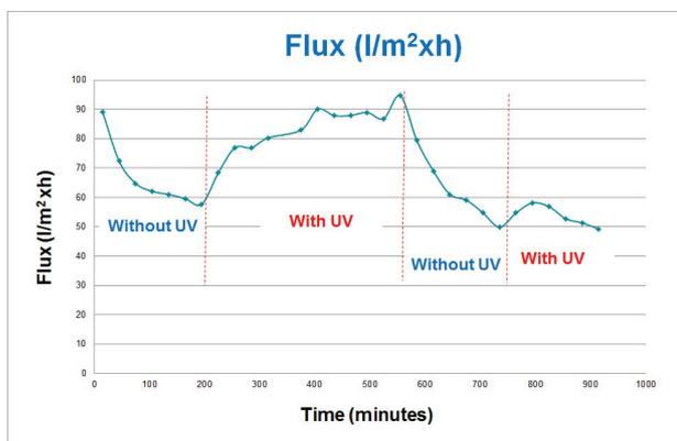
Flux in cross-flow filtration as a function of time and use of UV light.
