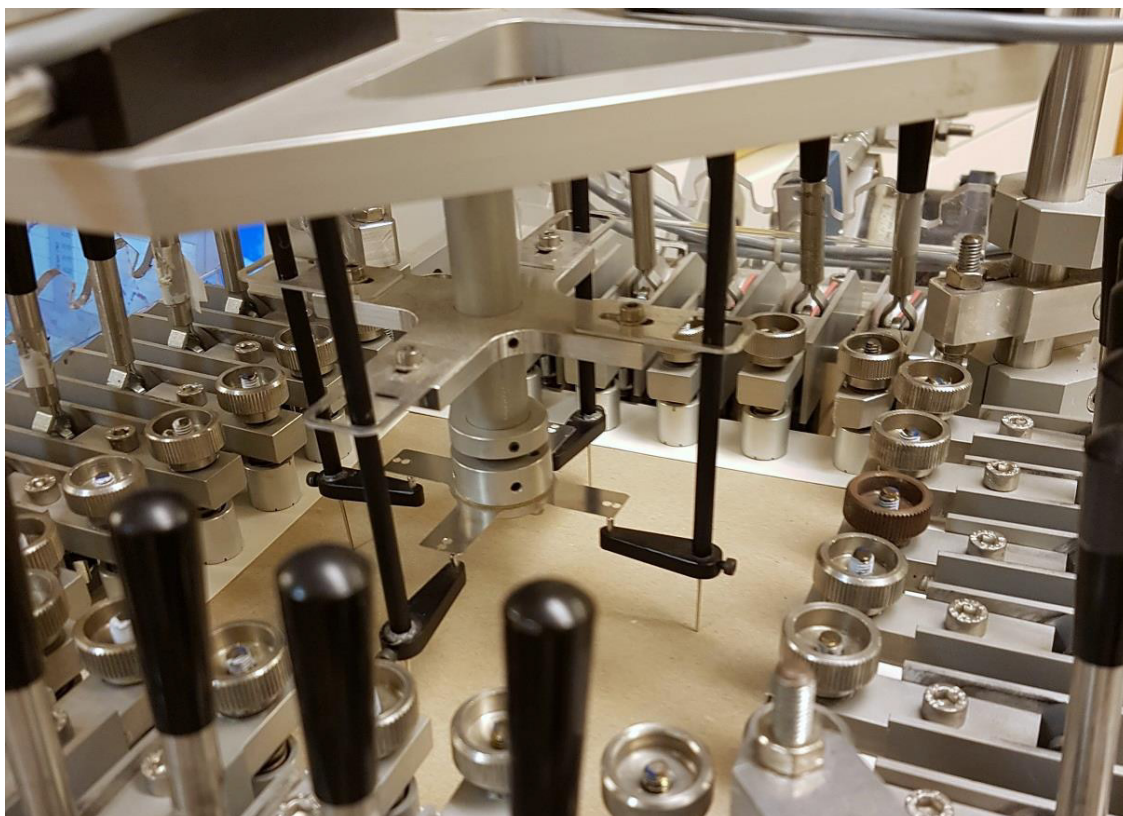
Figure 3. The bi-axial dryer instrument available at RISE. Stresses and strains are prescribed and/or recorded in the two directions of the sheet. The instrument was recently upgraded with continuous NIR-based measurement of the sheet dryness.
