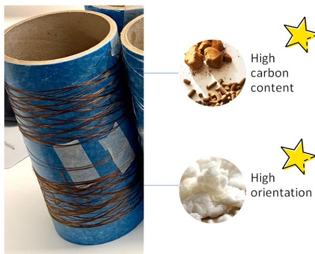
**Figure 1.** Wet spun cellulose-lignin yarn that can be used as a carbon fiber precursor. The lignin provides a high carbon content while cellulose provides high molecular mass and orientation.
