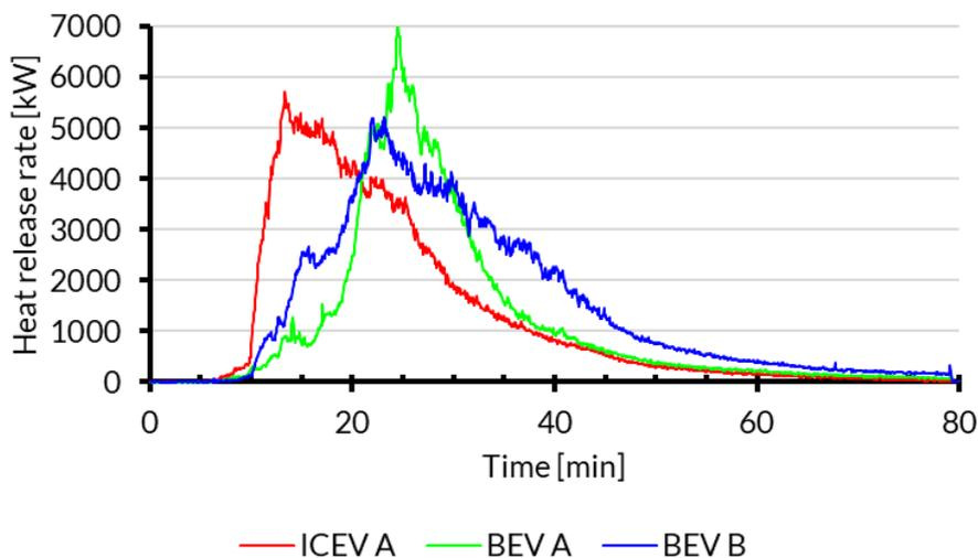
Figure 4. Heat release rate (oxygen consumption calorimetry) for the three vehicles.
