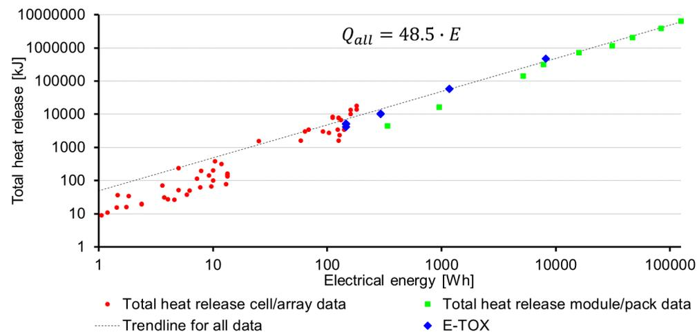
Figure 5. Total heat release data plotted with respect to the nominal electrical energy of the test objects.
