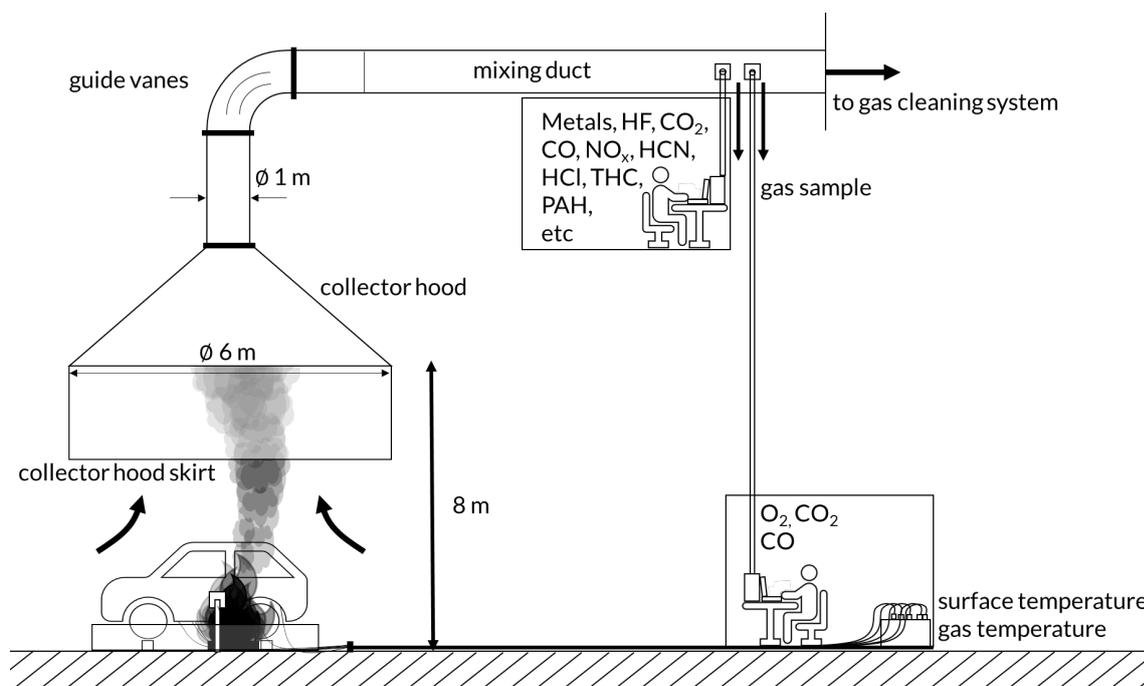
Figure 1. An overview of the test facility, test setup and measured data.
